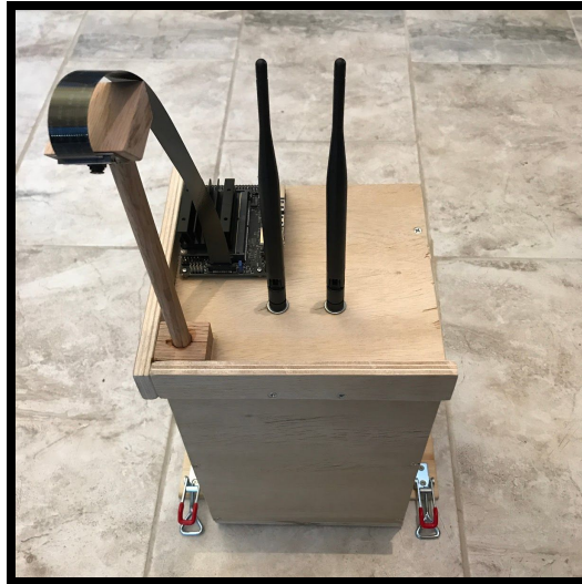
Figure-4.4.1: Camera and Jetson Nano mounted on top of HPEC building (mockup)
