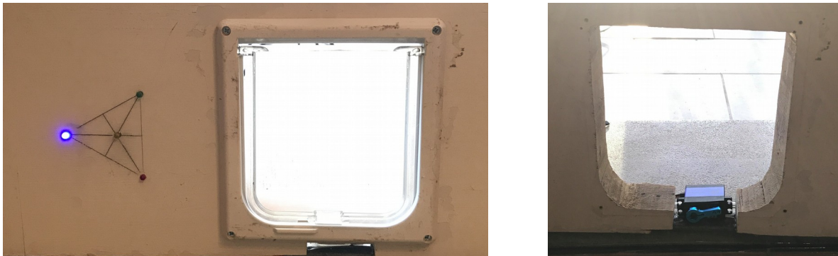
Figure-21: LED Implmentation (RHS) & Servo Latch Impmentation (RHS)
